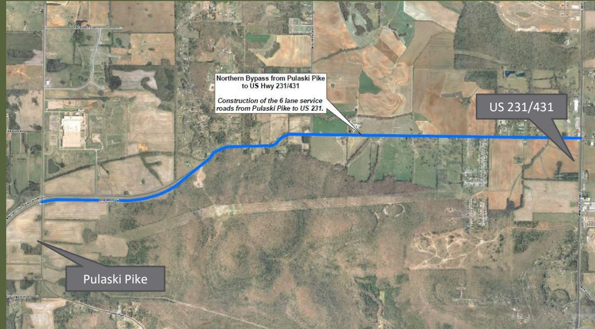
Status: Utility work close to completion. Contractor is working east to west. Grading work and drainage structure construction continues. Project approximately 70% complete.
